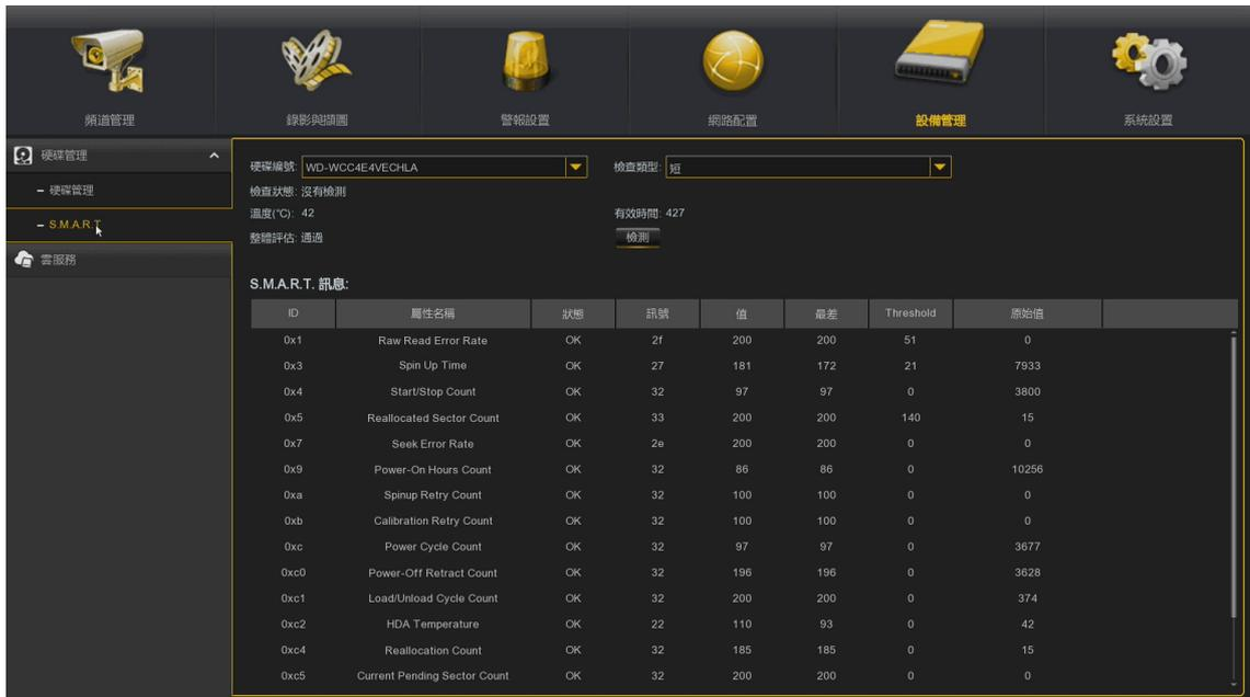
The screenshot shows the S.M.A.R.T. utility interface. At the top, there are navigation icons for Channel Management, Recording & Playback, Alarm Settings, Network Configuration, Device Management, and System Settings. The main area displays the drive model 'WD-WCC4E4VECHLA' and the test type '短' (Short). Below this, a table lists SMART attributes with their IDs, names, status, and various metrics.
