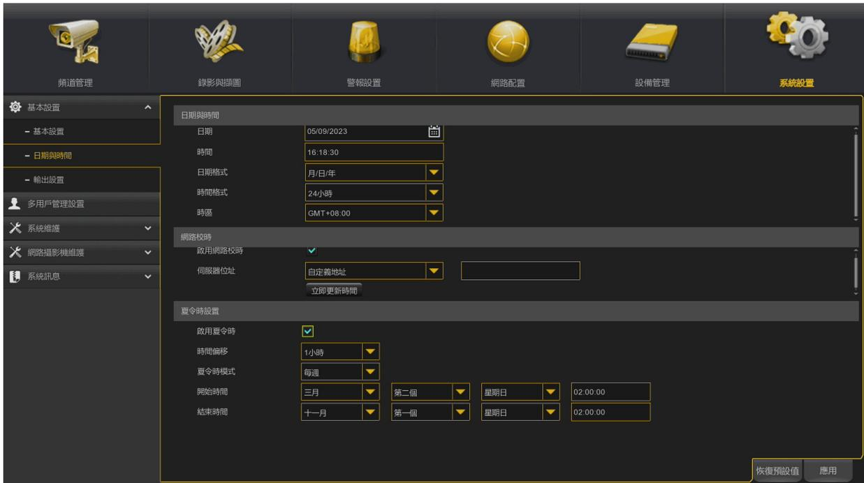
The screenshot shows a web-based system settings interface. The top navigation bar includes icons for Channel Management, Recording & Scheduling, Alarm Settings, Network Configuration, Device Management, and System Settings. The left sidebar lists various settings categories: Basic Settings, Date & Time, Output Settings, Multi-user Management, System Maintenance, Network Camera Maintenance, and System Information. The main content area is titled 'Date & Time' and contains several sections:
